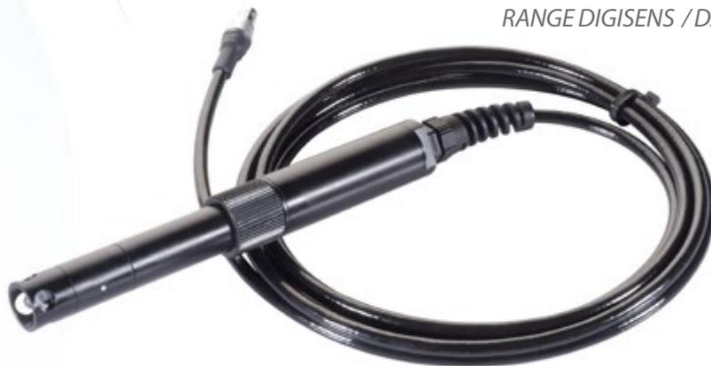
**The PHEH sensor has been designed to perform under hard conditions from pure mountains water with conductivity as low as 20  $\mu\text{S}/\text{cm}$ , lakes and rivers (100 – 2000  $\mu\text{S}/\text{cm}$ ), seawater with conductivities of 50 mS/cm and to wastewater with conductivity higher than 200 mS/cm.**
